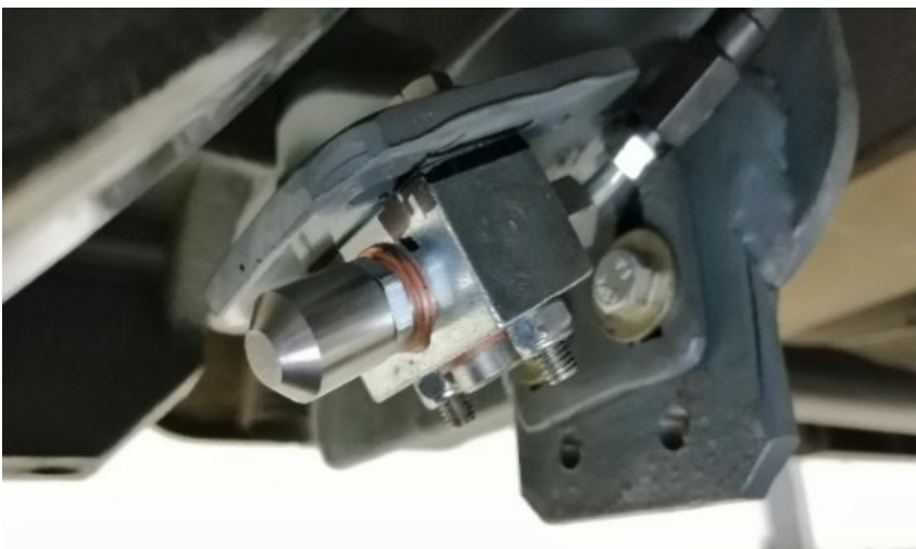
Spray nozzle for top of rail friction management and/or flange lubrication
